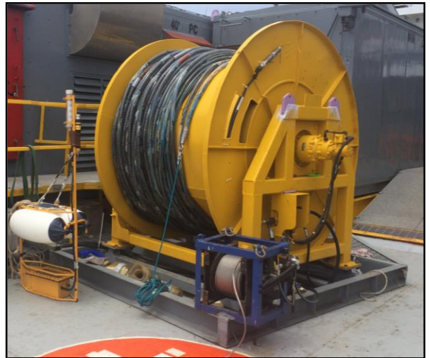
TTS Brevini Tugger winch mounted alongside TTS Streamer winch
